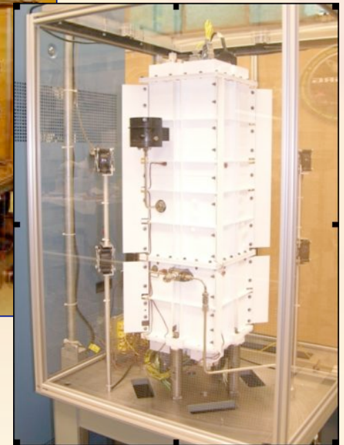
ASRG EU on test at NASA Glenn
