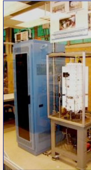
ASRG EU on test at NASA Glenn
